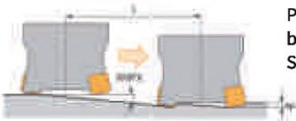
Please set the angle of ramping machining below RMPX.
